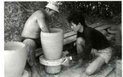
FIG. 11. TEAM OF POTTERS USING COIL-AND-THROW PROCESS TO MAKE SERIES OF STONEWARE JARS. NONG KHAI PROVINCE, NORTHEAST THAILAND, 1990
