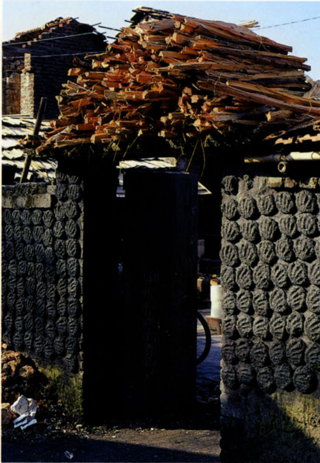
■ Figure 8. A gateway to a pottery workshop in Bat Trang supporting a bundle of firewood. On the walls are dry cakes of coal dust mixed with clay, used as fuel in the kilns.
