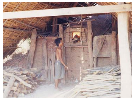
Fig. 27. Kiln at Mudon near Moulmein, Burma (Myanmar), showing uppermost firehole of three being used.
