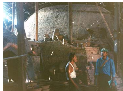
Fig. 28. Twentieth-century jar kiln at Twante, Burma (Myanmar), with a firing chamber nearly five meters high.
